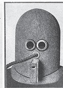
The above photograph shows a close-up view of the Isolator helmet. The oxygen supply enters the helmet via the tube shown.
